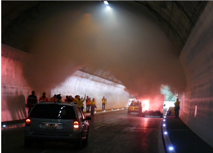
Figure 20: Hot smoke test in a road tunnel
