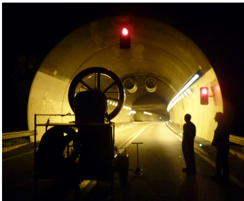
Figure 16: Mobile jet fan at tunnel portal for simulations of external pressures
