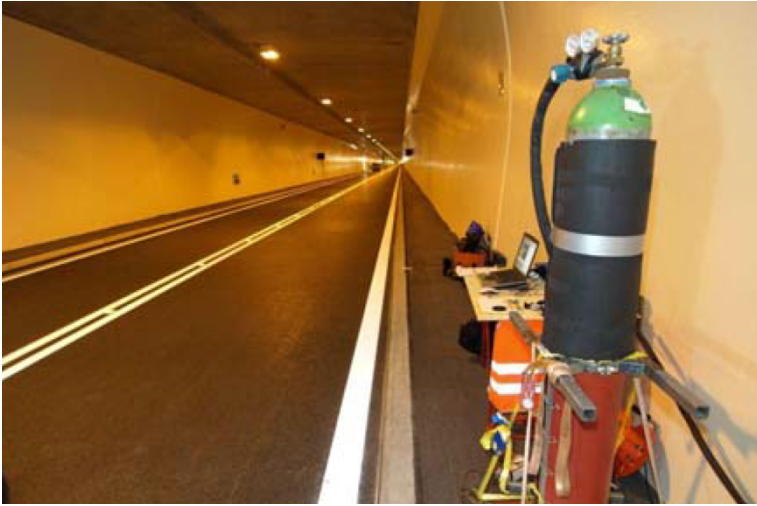
Figure 12: Tracer Gas injection in a road tunnel
