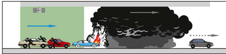
Figure 8. Smoke movement in a tunnel with unidirectional traffic without exhaust
