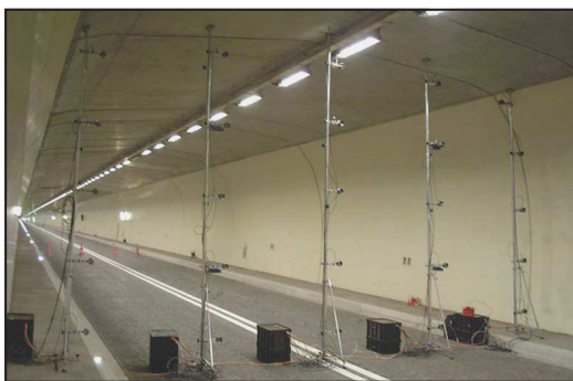
Figure 12. Grid measurement for calibration of anemometers (according to ISO 5802)
