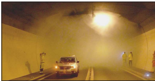
Figure 7. Front of smoke area under outermost open exhaust damper
