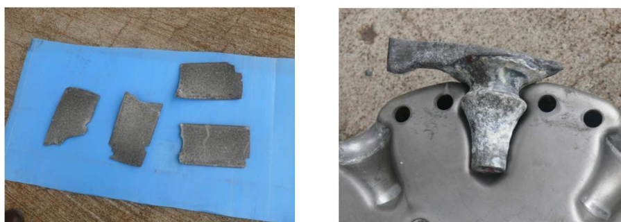
Fig 1 damaged jet fan: broken blades parts (left), blade foot (right)
