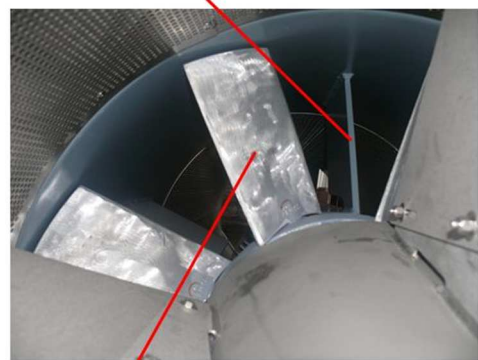
Forced vibration of rotating blades by n_2 struts
