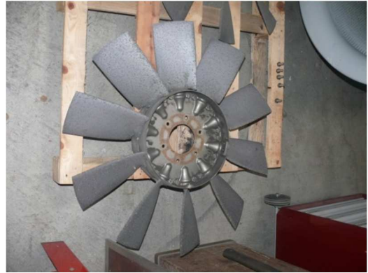
Fig 2 : undamaged wheel of a jet fan
