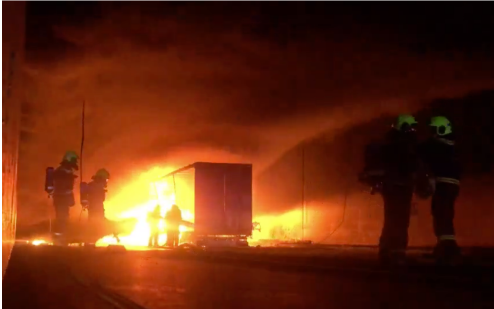
6 7 Figure 2 Fire fighting of a large tunnel fire under controlled flow conditions 8
